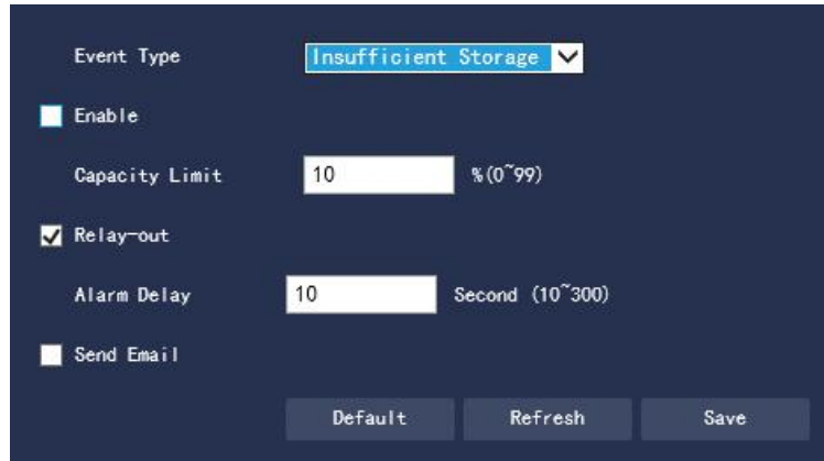
Figure 3.4-7 Insufficient Storage Space Warning
